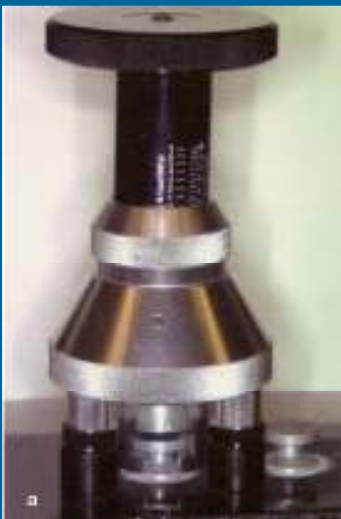
a) Testing apparatus for pull off strength c) Pull off strength results over wet concrete with BDC Vapor Seal
